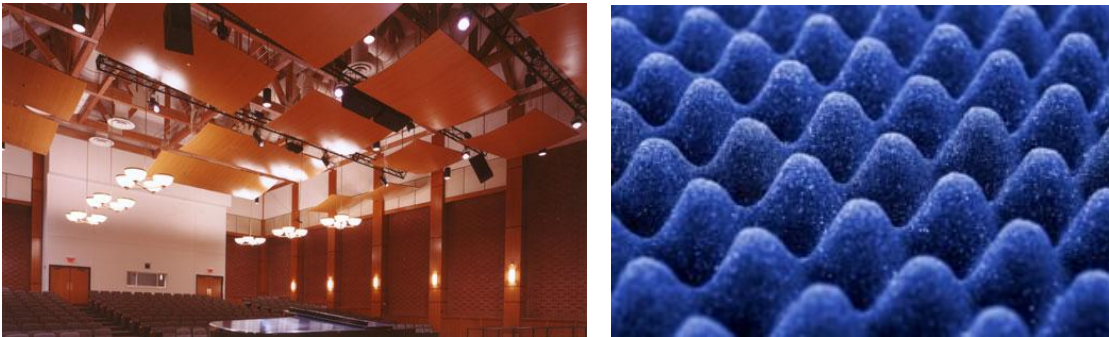
Hard surfaces are sound reflectors (left); soft surfaces are sound absorbers (right)
